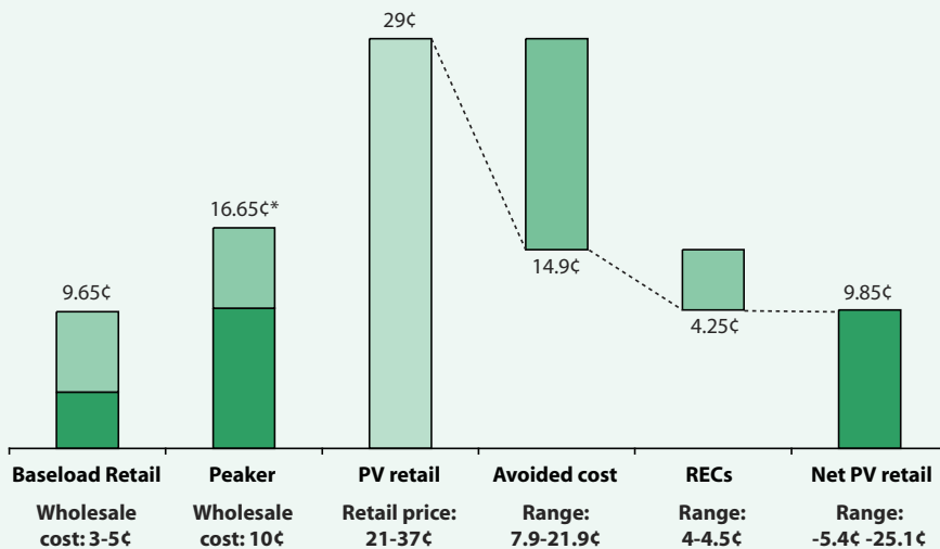
Figure 2. Illustrative price and cost comparison of conventional and solar electricity generation (assumes midpoint values for ranges)
